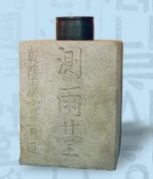
"Chukwookee", Korea's first standardized rain gauge invented in 1441, one of the earlies! instrumental measurements in the world
